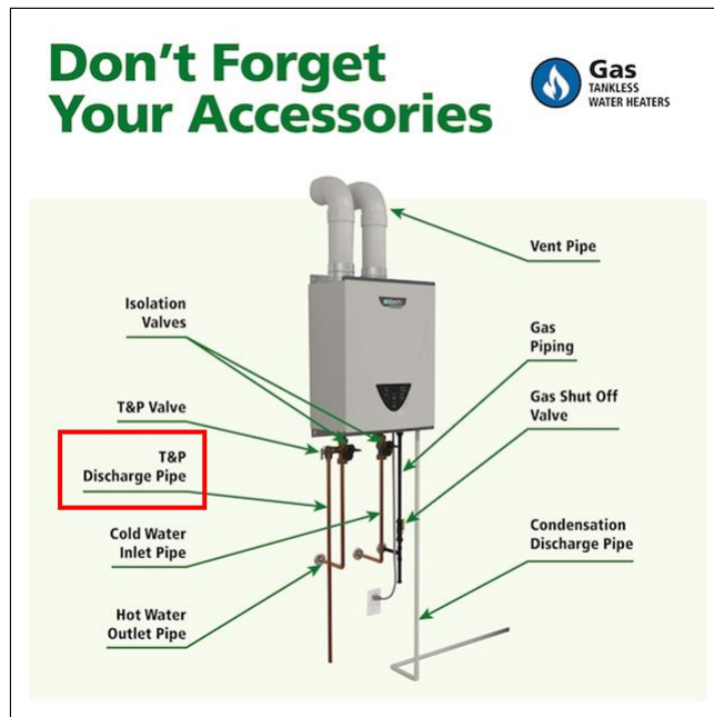
3.6 Item 3(Picture) Example of water heater with discharge pipe
